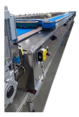
By positioning the satellite transfer device up- and down the DLms track, off-line conveyor length can be converted into an extension of the in-line buffer. Given this unique feature, our DLms cannot only be used as a metering device, but also as a stand-alone accumulator to prevent starvation of downstream equipment. It is commonly used as empty buffer to run-empty machines, but also as filled buffer behind e.g. a depalletizer.
