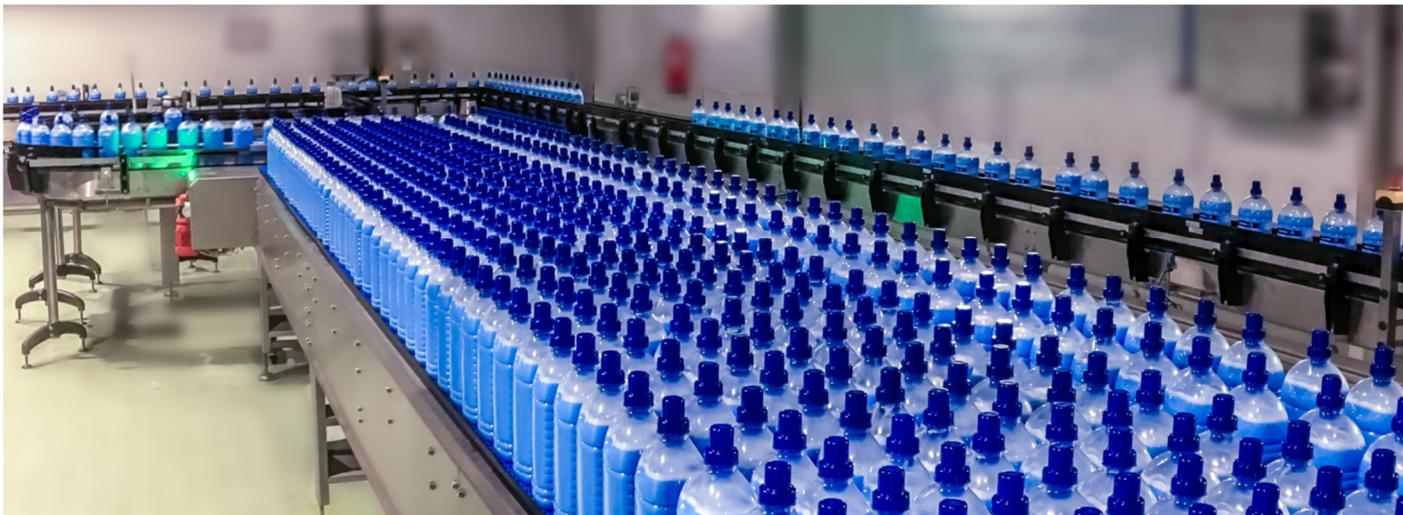
**FTms HORIZONTAL MULTILANE FIFO ACCUMULATOR**
